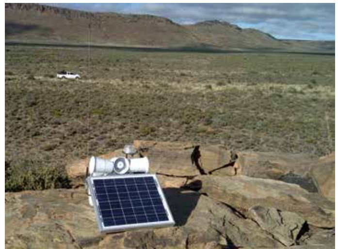
Figure 6.2. Solar powered acoustic and light generating device ( \approx frightening device) set on a livestock farm in South Africa. Photo: Niel Viljoen.
